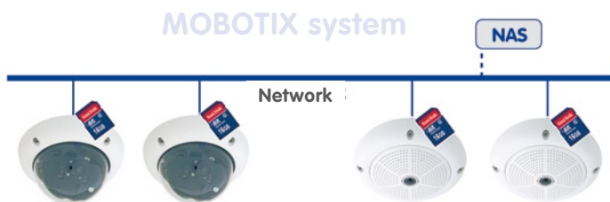
Software and storage integrated in the MOBOTIX camera
